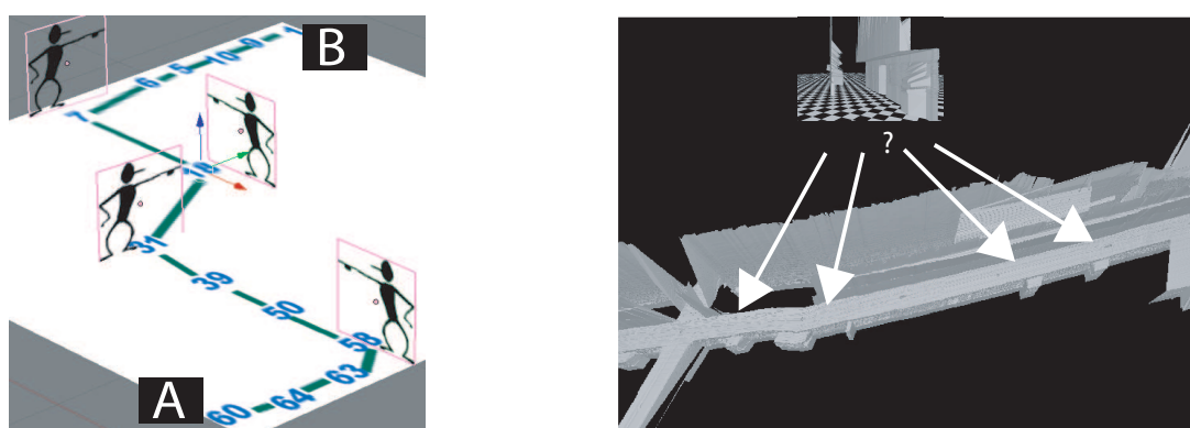
Figure 4.2: The robot is led through the environment on the Environment Familiarisation run, left. The 3D point clouds must be registered in the environment, right.
